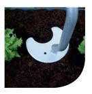
Disc profile and synchronisation setup is designed to maximise cultivated area and provide adequate tolerance to plant misalignment, in order to minimise crop damage. The tolerance required depends on the growth habit of the crop plants. For crops with regular growth habits the uncultivated area can be very small. 80mm D uncultivated plant zone is common.
