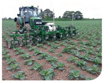
Robocrop InRow can continue to function even if some plants have grown into one another however for good reliable operation good plant separation is important
