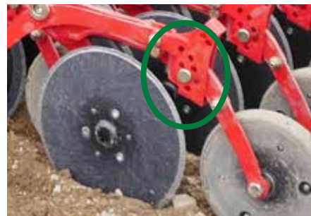
Flexible press wheel setting
