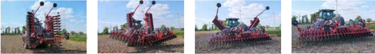
Automatically steered folding sequence of power harrow and coulters bar increase drivers comfort.
