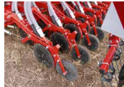
CX-II coulters with double entry for two sorts of application and seeding in one pass.
