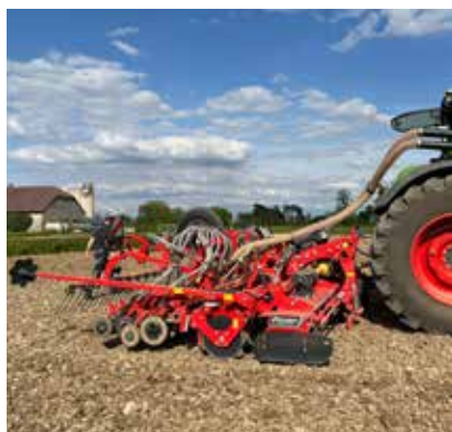
Solo power harrow operation at the headland is made possible by the ability to lift the coulters bar.
