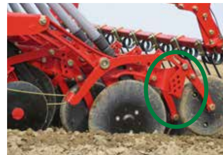
Lifted press wheel setting
